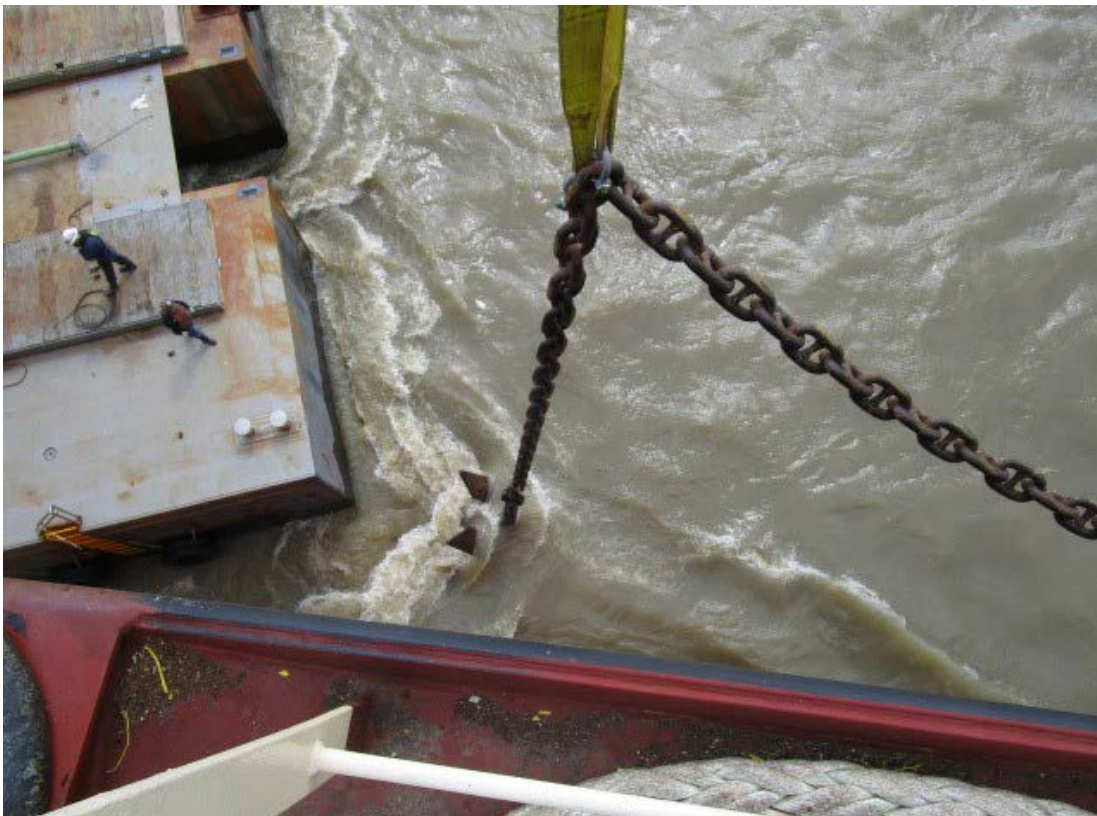
Figure 9 | Floating crane barge assistance in recovering an anchor
