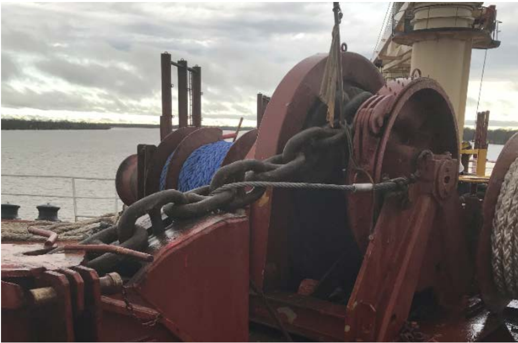
Figure 7 | Proper securing of the anchor chain with disengagement of the gear reduces the risk of winch or motor damage
