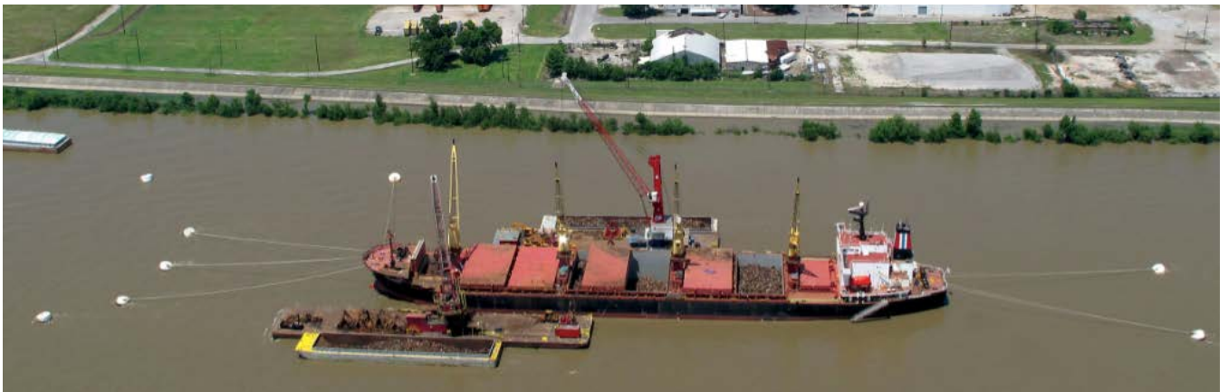
Figure 4 | Midriver three-point mooring at bow, two point mooring astern
