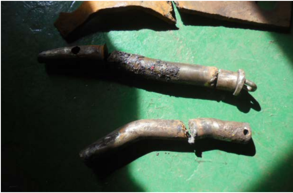
Figure 3 | Failed stopper pins from the anchor windlass guillotine stopper
