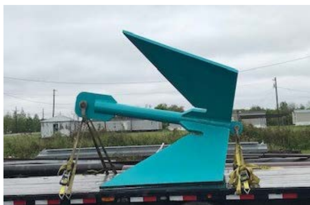
Figure 10 | Typical grapple hook used for anchor recovery
