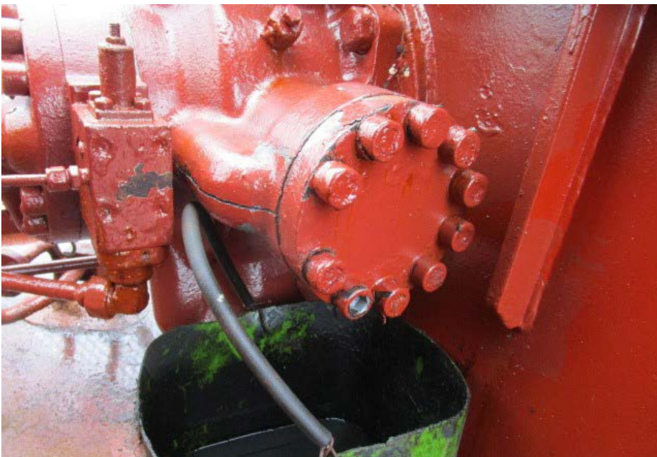
Figure 2 | Ruptured motor housing to windlass experienced during attempted recovery of anchor
